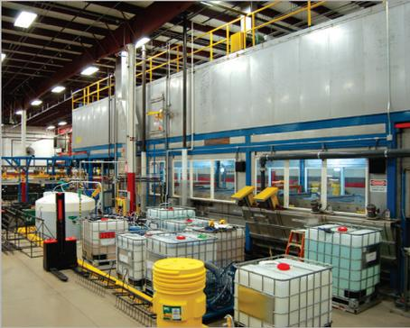
TTX also coordinates the integration of environmental rooms that provide optimal conditions for powder application and storage. In addition, TTX Environmental offers complete wastewater treatment systems and reverse osmosis equipment that can be incorporated into your system to provide high quality tank makeup and rinse water.
